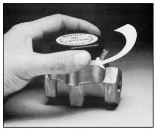
Keeping the tool face parallel to the OSV cover, carefully rotate the tool and gently press on the OSV cover. NOTE: It is important not to press the tool too tight. Minimum pressure will hold the tool in place while priming the fuel pump.
