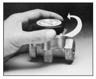
To remove the OSV tool, again carefully rotate and lift straight off the OSV valve. Keep the tool face parallel to the OSV cover.
