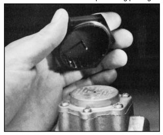
Carefully position the tool stem perpendicular to the OSV cover and above the OSV breathing hole. Gently insert the stem through the breathing hole until the tool stem touches the OSV diaphragm plate.
