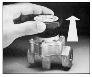
CAUTION: As soon as priming is complete make sure the OSV tool hase been removed.
